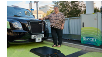
◀ Wireless Charging of Electric Taxis (WICET): The UK's first wireless charging electric taxi demonstration in Nottingham.
