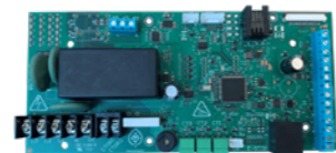
◀ This AC charge controller, for single- or three-phase EV chargers, interfaces with control boards such as the one pictured above to support smart charging.
